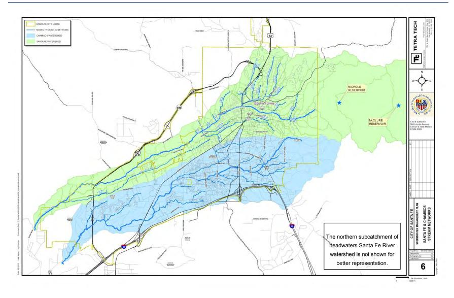
*Figure 6.* Stream networks selected for hydraulic modeling inside XPSWMM.
