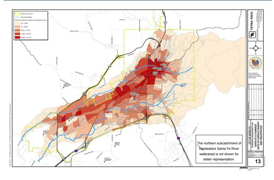
*Figure 13.* Ratio of LSPC simulated surface runoff to precipitation for the Santa Fe River and Arroyo de Los Chamisos watersheds.
