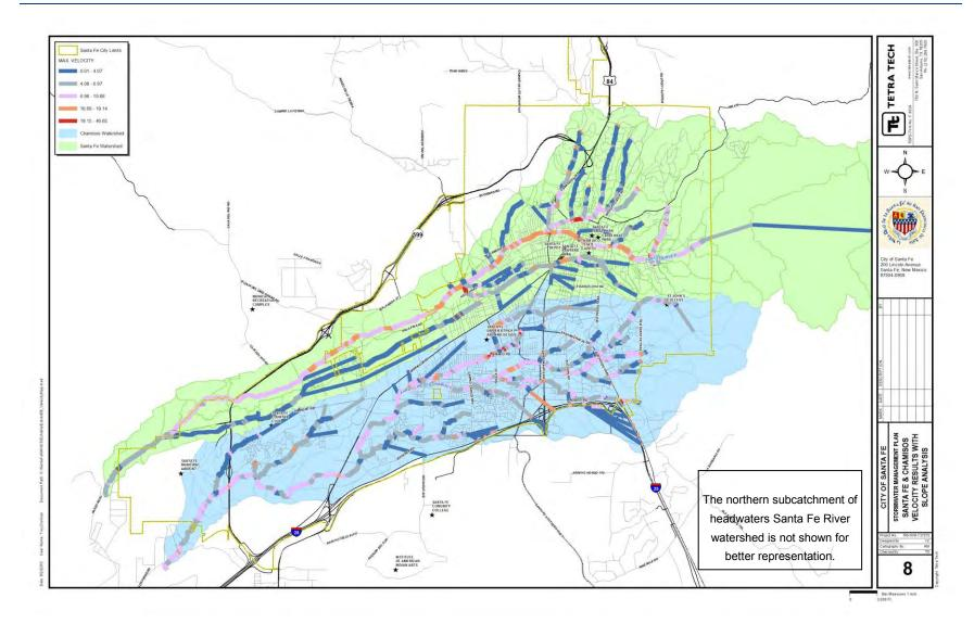
Figure 8. Maximum velocity in reach segments.
