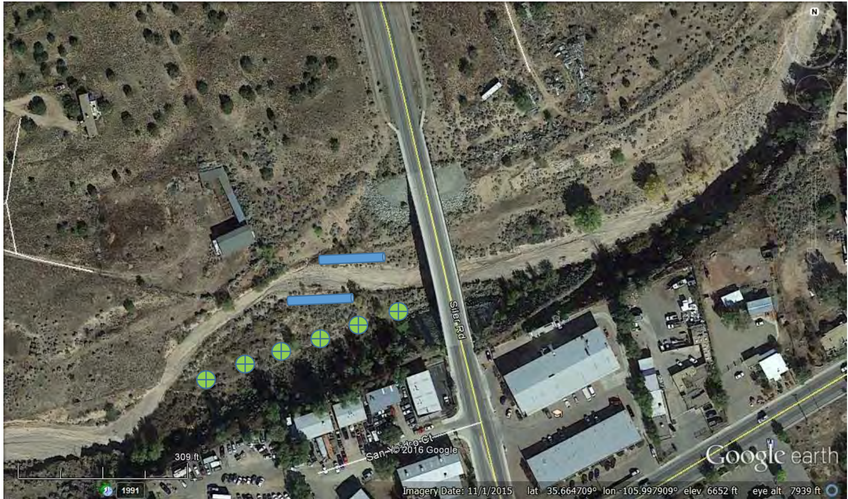
Figure 2. Aerial photograph showing Siler Rd crossing the Santa Fe River. Conceptualized piping that distributes discharged water are shown as blue bars. Conceptualized bank of infiltration galleries is shown as green markers.
