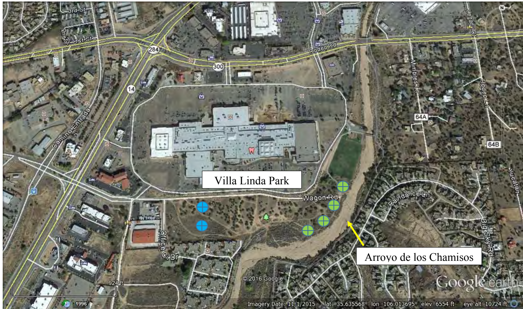
Figure 3. Aerial photograph showing Villa Linda Park and Arroyo de los Chamisos. Conceptualized bank of infiltration galleries is shown as green markers. Conceptualized recovery wells are shown as blue markers.
