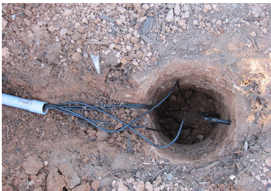
Figure 2. Decagon 5TM soil moisture probes inserted into an Alire Loam soil profile at 6 inch intervals below the soil surface.
