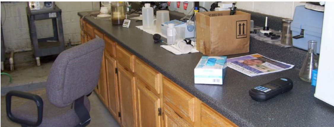
Mini Laboratory. The operators run various in house process control tests in the DAF (Dissolved Air Flotation) Mini Laboratory. This allows the operators to check how the plant is performing and make any necessary changes.
