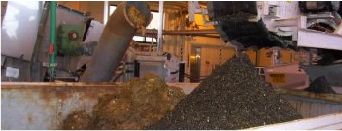
After dewatering they are discharged to the hoppers or dumpsters placed under the chutes.
